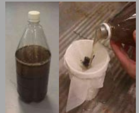
Fig 3 (left). Fill bottle with water to this level. Fig 4 (right). Pour light fraction through handkerchief filter.
